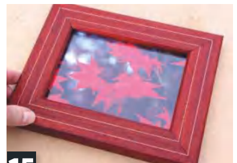
15 Insert glass followed by the photo. Either pin or clip the backing board into the rebate and attach hooks or a flap
